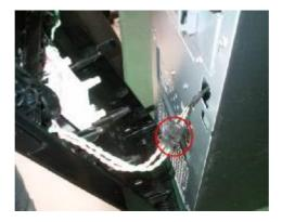
7.2 Insert three hooks to chassis in right side and Clasp three hooks in left side
